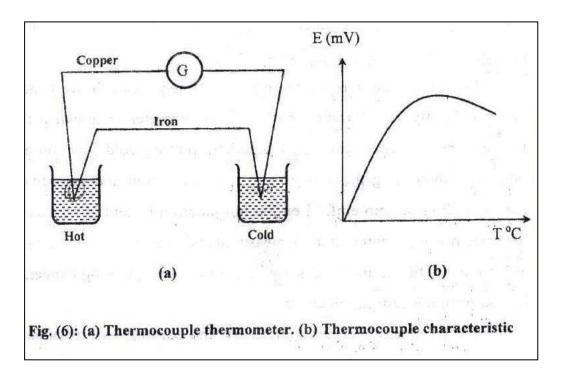
It has been found that for temperature up to 300°C, copper constantan and iron constantan are good as they give thermo emf of the order of 40 to 60 microvolt per degree temperature difference between junctions.
