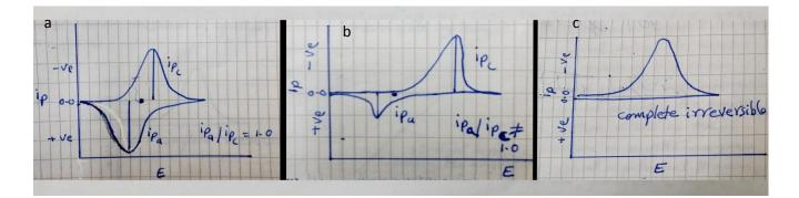
However, in case of irreversible processes, the peak current can be related to the sweep rate using the following equation:  $i_p = 3.01 \times 10^5 n (\alpha n_a)^{1/2} A C D^{1/2} v^{1/2}$
